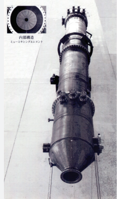
VOC Stripping Tower
